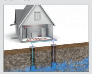
A groundwater heat pump collects energy from the groundwater. The water is pumped up from a water borehole to a heat exchanger, where the energy is recovered.
