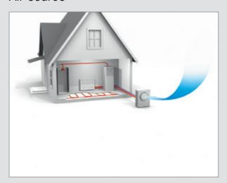
With an air source heat pump there is no need to dig or drill. Instead the energy is sourced straight from the surrounding air.
